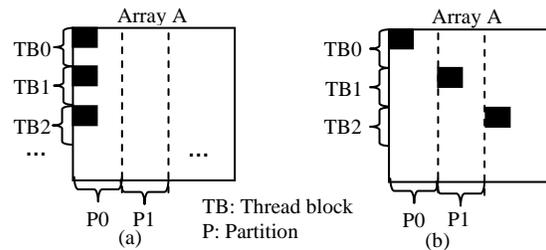
Figure 9. Eliminating partition camping. (a) Accesses to array A resulting in conflicts at partition 0. (b) Adding an offset as ( $partition\ size * bidx$ ) eliminates the conflicts. The dark regions represent the memory footprint of  $A[idx][0]$  from different thread blocks.
