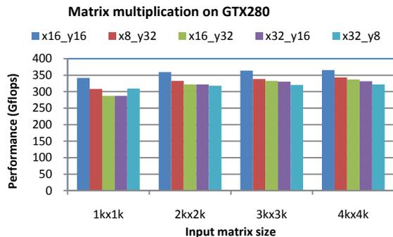
**Figure 10.** The performance impact (GTX 280) of the number of merged threads/thread blocks. ‘ $xN_yM$ ’ means that  $N$  thread blocks merged along the X direction and  $M$  threads merged along the Y direction.
