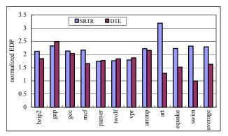
Fig. 7, Normalized Energy-Delay Product relative to single-thread execution.
