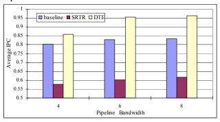
Fig. 5, Performance impact of pipeline bandwidths.
