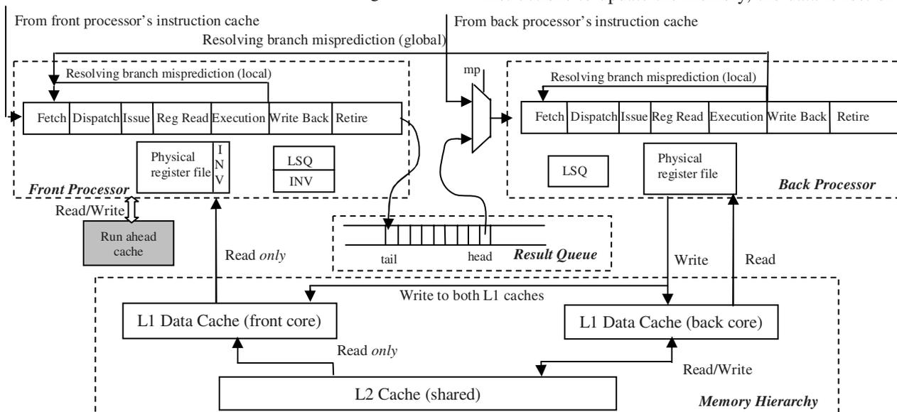
Figure 3. The design of DCE architecture.
