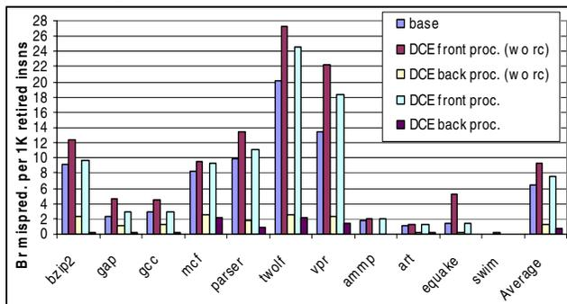
**Figure 5. Branch mispredictions detected in a single baseline processor, the front and back processors in DCE with and without a run-ahead cache. (some numbers are too small to be discernible, e.g., the misprediction rate at DCE back proc. for *ammp*)**
