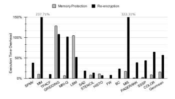
**Figure 1.** Execution time overheads of memory security with a state-of-the-art scheme (PSSM [27]) and domain crossing re-encryption overheads. The former was collected from GPU simulation with machine configuration from [27], while the latter is from a real machine described in Section 5.
