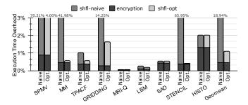
**Figure 7.** Kernel execution time overheads of naive LITE (shfl-naive+encryption) vs. optimized LITE (shfl-opt+encryption) over unsecured GPU baseline on regular GPU benchmarks.
