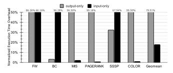
**Figure 10.** Normalized execution time overhead over full encryption of optimized LITE for input-only encryption vs output-only encryption on irregular GPU code.
